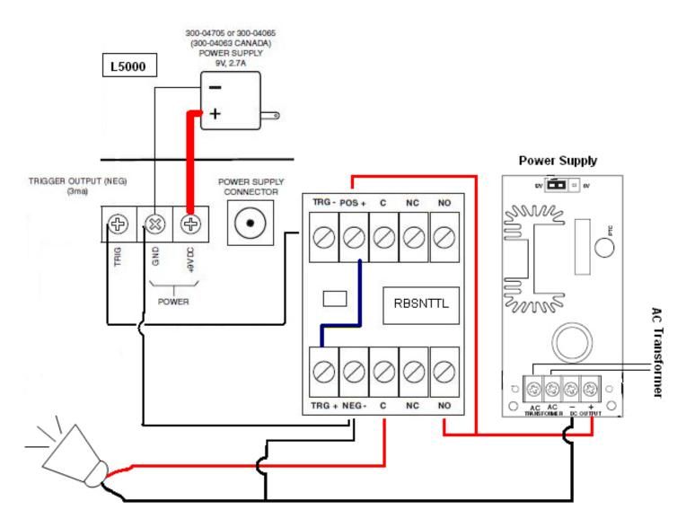
Due to the 3mA current limit of the L55200/L7000 output trigger, the Altronix TTL Sensitive relay must be used. A jumper wire is required from TRG+ to the POS+ terminal, as well as a common ground.
