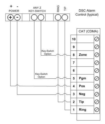
DSC Control Wiring & Key-Switch Option
