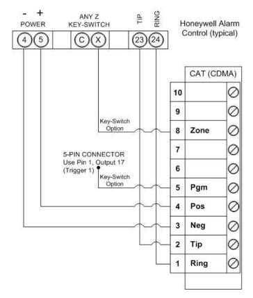
Honeywell Vista Control Wiring & Key-Switch Option Note: Key-Switch programming is available for Vista-15 and up.
