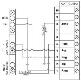
GE Control Wiring & Key-Switch Option
