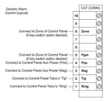
For basic Key-Switch operation with the Cellular CAT, the following alarm panel wiring is needed.
