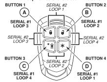
Using a Button: To activate a programmed function, press and hold the appropriate buttons for at least one second or more. The LED
