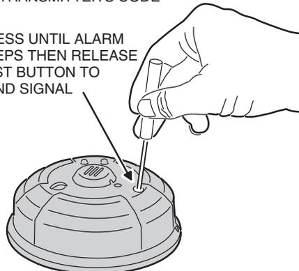
A TEST SIGNAL WILL BE SENT A FEW SECONDS AFTER THE SWITCH IS RELEASED
