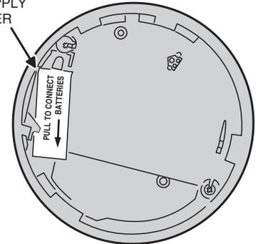
3-VOLT LITHIUM BATTERY - TYPES: DURACELL DL123A, PANASONIC CR123A, SANYO CR123A, ADEMCO 466. AVAILABLE AT LOCAL RETAILERS AND INTERNET SUPPLIERS. **NOTE: USE ONLY THESE SPECIFIC BATTERY MODELS.**
