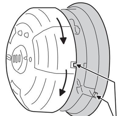
ALIGN TAB IN PLATE WITH NOTCH IN COVER
