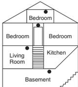
FIGURE 2. RECOMMENDED CO ALARM PLACEMENT FOR MULTI-LEVEL RESIDENCE
