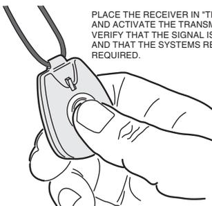
PLACE THE RECEIVER IN "TEST" MODE AND ACTIVATE THE TRANSMITTER. VERIFY THAT THE SIGNAL IS RECEIVED AND THAT THE SYSTEMS REPORTS AS REQUIRED.
