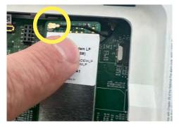
Push the IQ Card firmly into place. Connect the PowerG antenna jumper to the daughter card.
