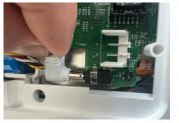
Once the IQ Panel has completely powered down, unplug or disconnect the power by removing the barrel jack connector inside the panel or by unplugging the power supply. NOTE: it is NOT required to disconnect the battery.
