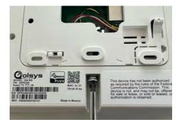
From the bottom of the panel, find the retaining screw, loosen completely.
