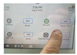
Run the "PowerG" test. Allow up to 2 min for the panel to successfully test the radio in the new IQ Card. If test fails, reboot the panel and try again.
