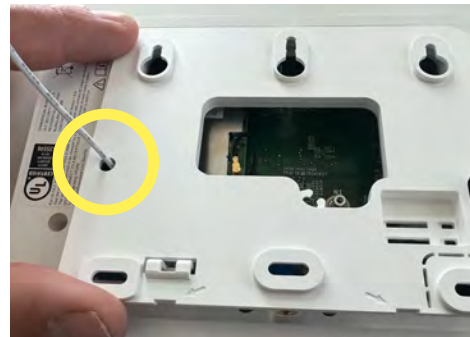
Ensure the white SRF antenna is routed out the hole in the backplate. Press down on the bottom and tighten the retaining screw.
