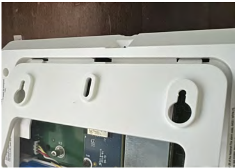
Replace the back cover, top tabs first.
