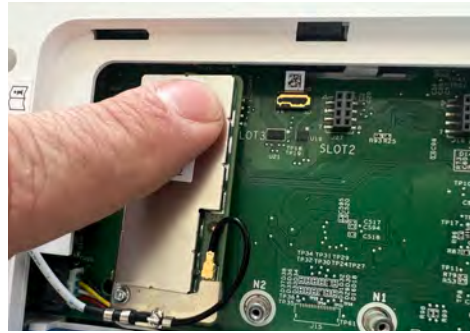
Push the IQ Card firmly into place.
