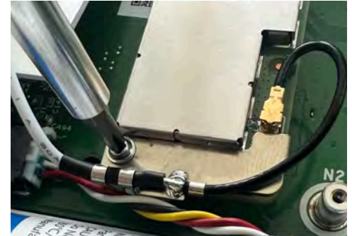
Install and tighten the provided locking screw to secure the IQ Card into place. Ensure the antenna remains connected and does not interfere with the battery.
