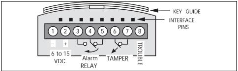
Figure 3.1: Wiring to terminals
