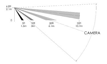
The following image is the PIR Lens Coverage from the top view. The camera coverage area is narrower than the PIR coverage area. When installing, mount sensor where subjects are likely to be centered in or across PIR and camera field of view.
