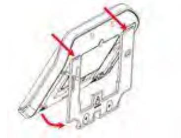
Align the UltraSync panel to the top clips on the wall bracket, then slide the panel into place so it sits flat against the wall.
