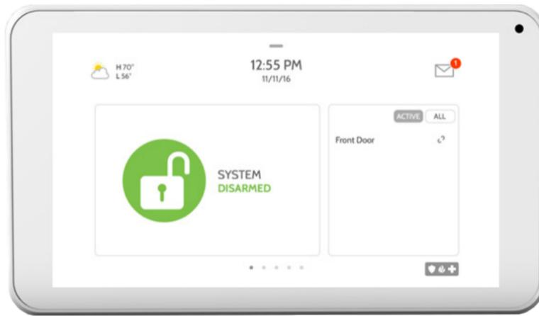
The IQ Remote is a 7" secondary tablet that can be installed to create additional access to the IQ Panel 2. You can pair up to three (3) of these tablets with the IQ Panel 2.
