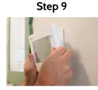
Tilt panel upward onto back plate until it snaps in place
