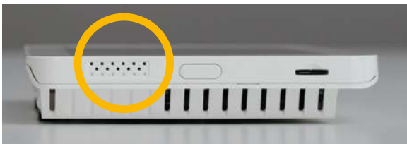
Speakers are located on each side of the panel
