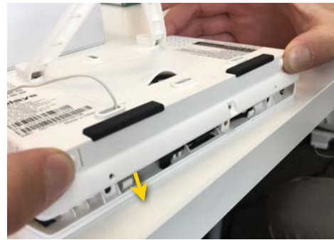
Replace the back cover, taking care not to pinch any antennas or wires.
