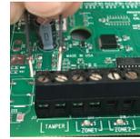
Trip the module by opening the tamper switch or by removing jumper installed in Step 1 from the "Tamper" terminals, then replace
