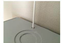
*If mounting inside a metal can, the antenna must extend outside the enclosure to ensure RF communication*
