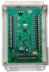
The IQ Hardwire 16-F offers a cost effective way of integrating hardwired security & smoke detector zones with the IQ Panel 2. It includes backup battery charging, 500mA of 12volt auxiliary power, an onboard siren relay, built-in status LED's for each zone and support for up to 10 two-wire smoke detectors. Normally Open and Normally Closed contacts are supported as well as powered zones like motion sensors and glass break detectors.
