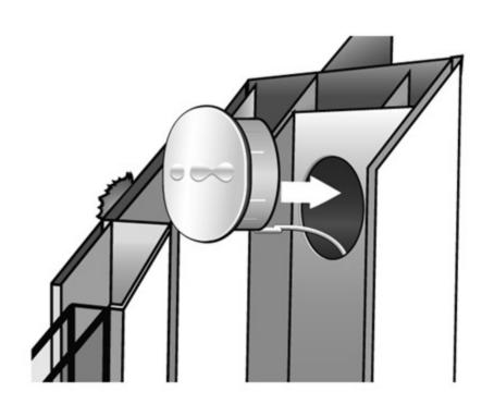
Insert the 5800MICRA's antenna into the extrusion hollow then press the transmitter body into the corded opening.
